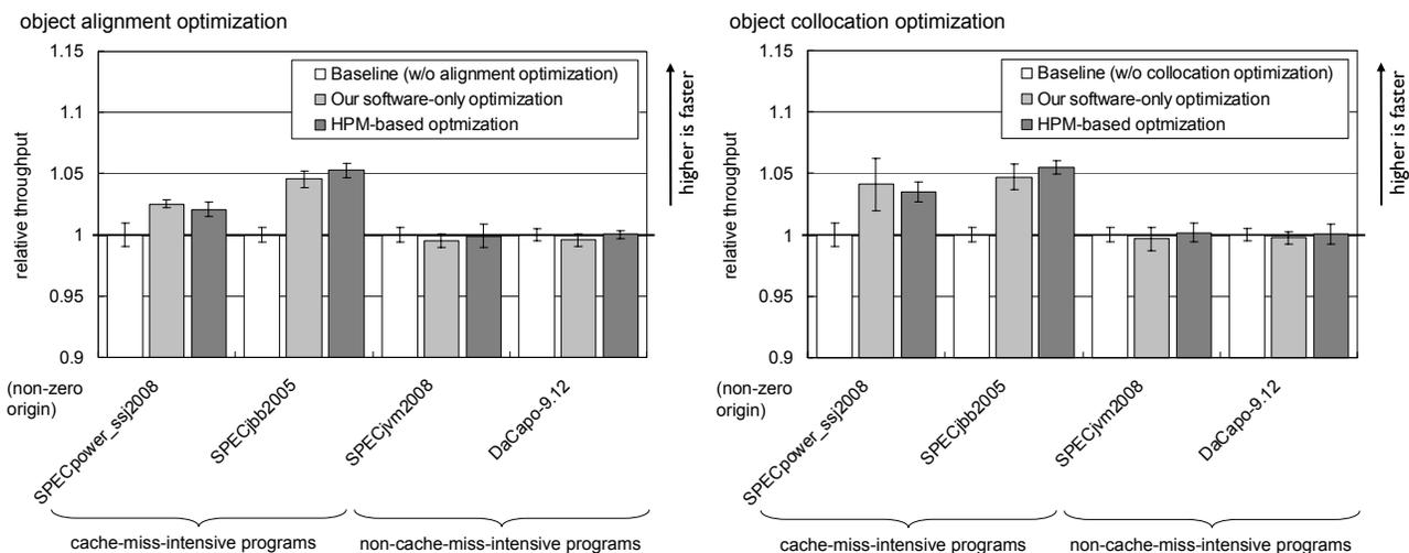
**Fig. 9.** Performance improvements from object placement optimizations with our approach and with HPM-based approach. The error bars show 95% confidence intervals. We used the Base threshold for pattern matching. Note that the origin of the Y-axis is not zero.
