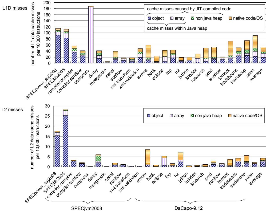
**Figure 4.** L1 and L2 cache miss ratios and breakdown by code location and access targets. We exclude the cache misses during stop-the-world garbage collection to focus on mutator performance.
