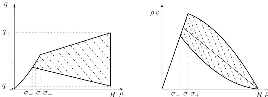
FIG. 3.2. *Newell-Daganzo standard flux function. Left: Fundamental diagram in state space coordinates. Right: Fundamental diagram in flux-density coordinates. The standard state is the usual triangular diagram. The congestion phase is two-dimensional (striped domain).*
