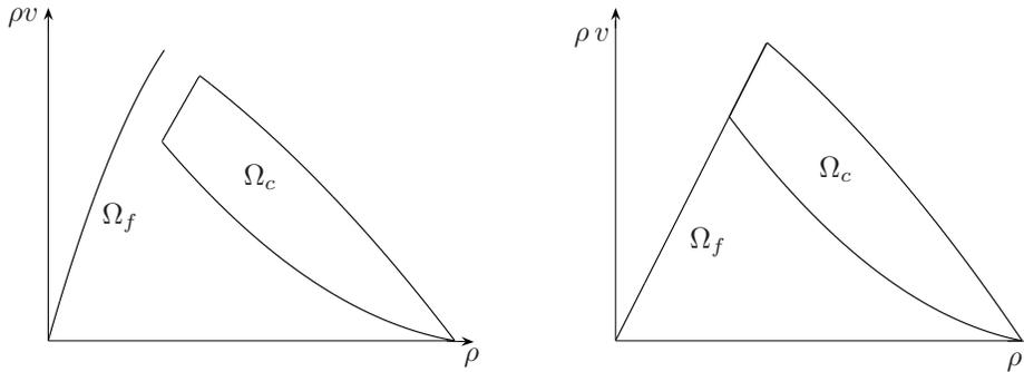
FIG. 3.3. *Different free-flow phases. Left: Fundamental diagram from the original Colombo phase transition model. Right: Fundamental diagram of the model derived in the present article in the particular case of a Newell-Daganzo standard state flux in the congestion phase.*
