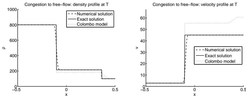
FIG. 4.1. *Exact solution (continuous line), computed solution (dashed line), and exact solution for the Colombo model (dotted line) for density (left) and speed (right). Between the two initial states, for the class of models presented in this article, appears a state  $u_m = (215.4, -0.03)$  which corresponds to the intersection of the 1-Lax curve going through  $u_l$  with the metastable phase. In this graph  $T = 0.4$  and  $\Delta x = 0.0013$ .*
