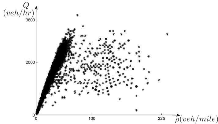
FIG. 3.1. *Fundamental diagram in density flux coordinates from a street in Rome. In congestion (high densities) the flux is multi-valued. Count  $C$  and velocity  $v$  were recorded every minute during one week. Flux  $Q$  was computed from the count. Density  $\rho$  was computed from flux and velocity according to the expression  $Q = \rho v$  (see [3] for an extensive analysis of this dataset).*
