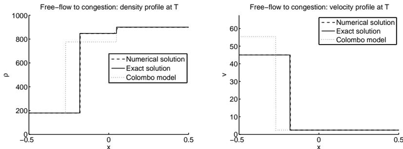
FIG. 5.2. *Exact solution (continuous line), computed solution (dashed line), and solution to the Colombo model (dotted line) for density (left) and speed (right). Between the two initial states appears a state  $u_m = (847.4, -0.24)$  which corresponds to the intersection of the lower bound of the diagram in congestion with the 2-Lax curve going through  $u_r$ . In this graph  $T = 1$  and  $\Delta x = 0.0013$ .*
