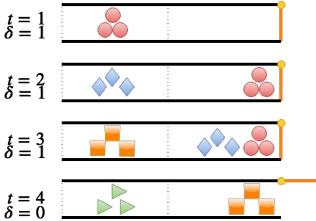
**Figure 3: Propagation model:** passengers move from left to right, passengers represented by the same icon entered the corridor at the same time. The corridor exit on the right-hand side can be open or closed.
