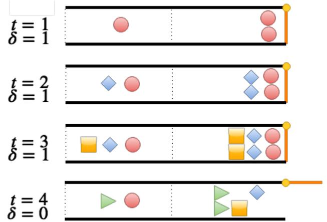
**Figure 4: Instantaneous model:** passengers do not move, only appear at a location and fade from the same location. Passengers represented by the same icon entered the corridor at the same time. The corridor exit on the right-hand side can be open or closed.
