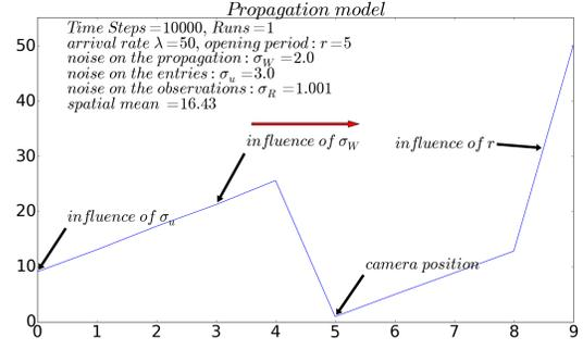
Figure 6: Local estimation error: for the propagation model with sensor placed in cell 5.
