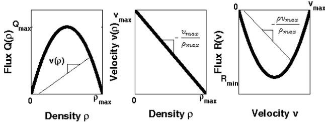
Figure 1. Greenshields model. **Left:** Classical fundamental diagram (parabolic). **Center:** Linear relation between speed and density. **Right:** Flux function for the LWR-v PDE (4). The flux is parabolic with negative values.
