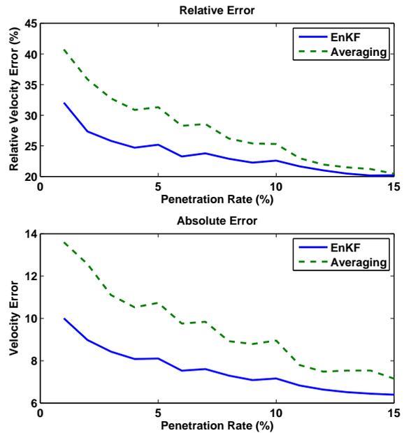
Figure 3. Error comparison of the EnKF CTM-v scheme (19)-(24) (solid) and the averaging scheme (25) (dashed) using Paramics. **Top:** Relative error computed from (26) as a function of penetration rate. **Bottom:** Absolute error computed from (27) as a function of penetration rate.
