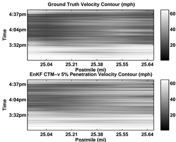
Figure 2. Paramics velocity contours. **Top:** Ground truth velocity contour average across all vehicles. **Bottom:** Estimated velocity contour from the EnKF CTM-v algorithm (19)-(24) at 5% penetration rate. X-axis: position along highway in postmile; Y-axis: time of day.
