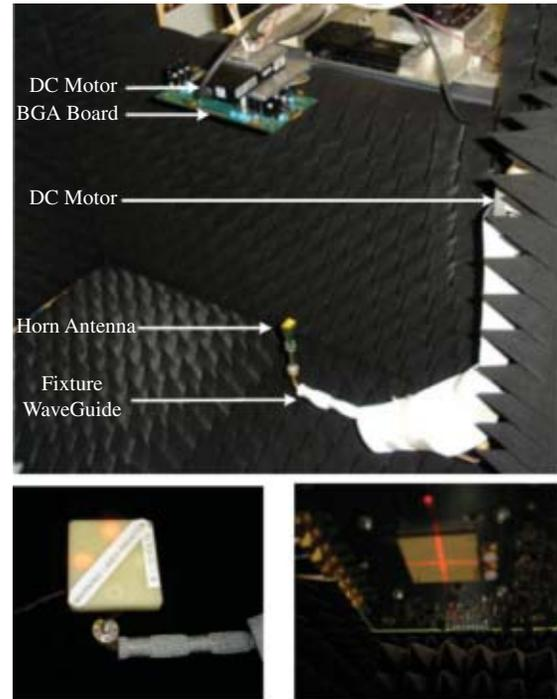
Fig. 11. Assembled module measured in anechoic chamber using automated testbed fixture.
