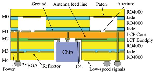
Fig. 1. Stack-up of the proposed flip-chip ball grid array (BGA) package.
