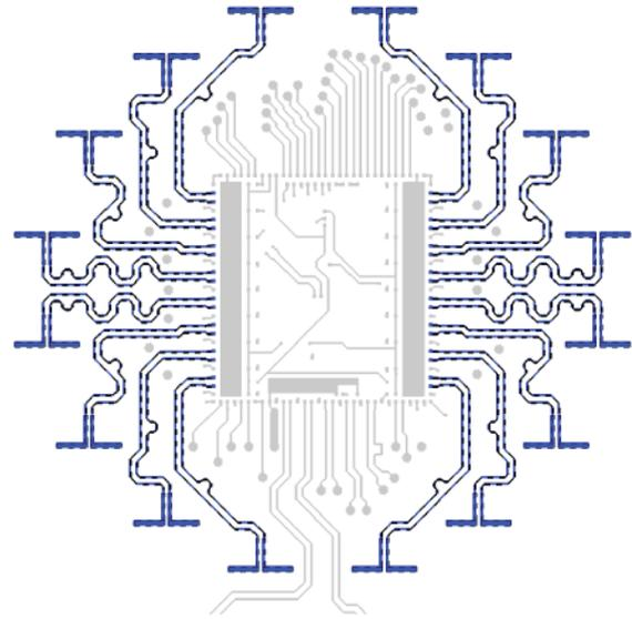
Fig. 2. Symmetric layout of 60-GHz interconnections (highlighted in blue) in Tx package.
