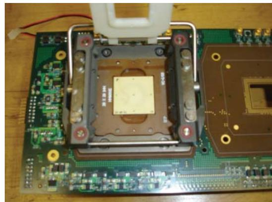
Fig. 8. Package mounted in test socket.
