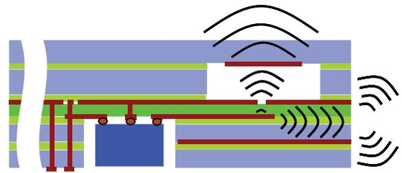
Fig. 14. Element-to-element antenna gain variation due to edge radiation.
