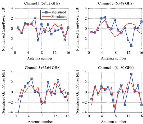
Fig. 12. Comparison of simulated and measured antenna gain of Tx package.
