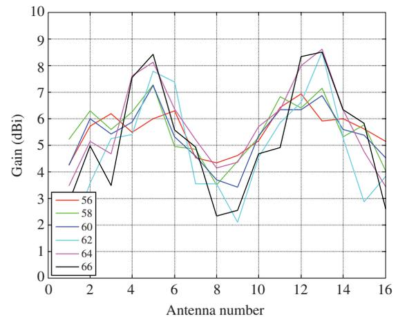
Fig. 5. Simulated antenna element gain at  $\theta = 0^\circ$  of, (top) Tx package (bottom) Rx package.
