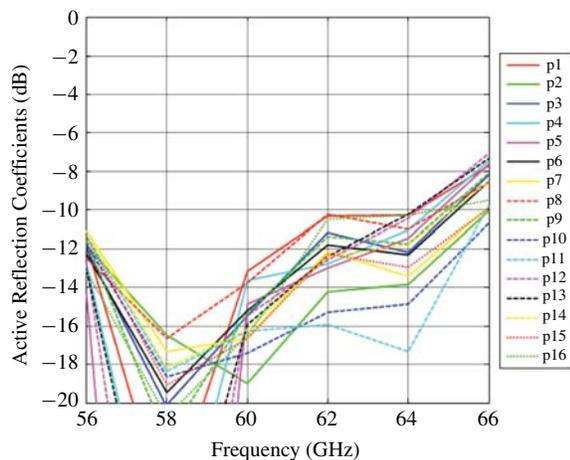
Fig. 4. Simulated reflection coefficients of 16 antennas in Tx package.
