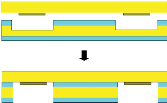
Fig. 13. Substrate and cavity manufacturing flow.
