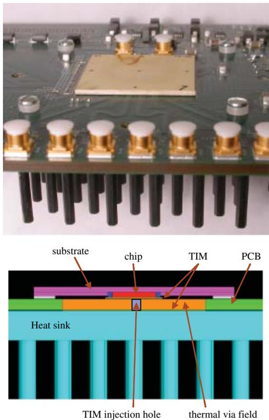
Fig. 9. Package mounted on evaluation board with heat sink.
