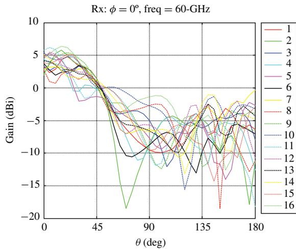
Fig. 6. Simulated array element pattern on the E-plane of Rx package.
