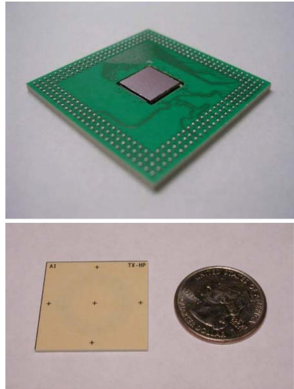
Fig. 7. First-of-a-kind multilayer organic package fully integrated with the 60-GHz phased-array IC.
