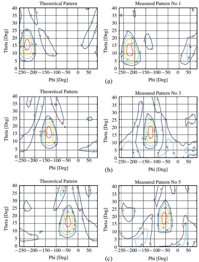
Fig. 15. 2-D, 16-element radiation patterns at 60.48-GHz in spherical coordinates for (a)  $\Theta = 18^\circ$  and  $\Phi = -225^\circ$ . (b)  $\Theta = 18^\circ$  and  $\Phi = -135^\circ$ . (c)  $\Theta = 18^\circ$  and  $\Phi = -45^\circ$ . Measured from a packaged Tx IC in an antenna chamber.
