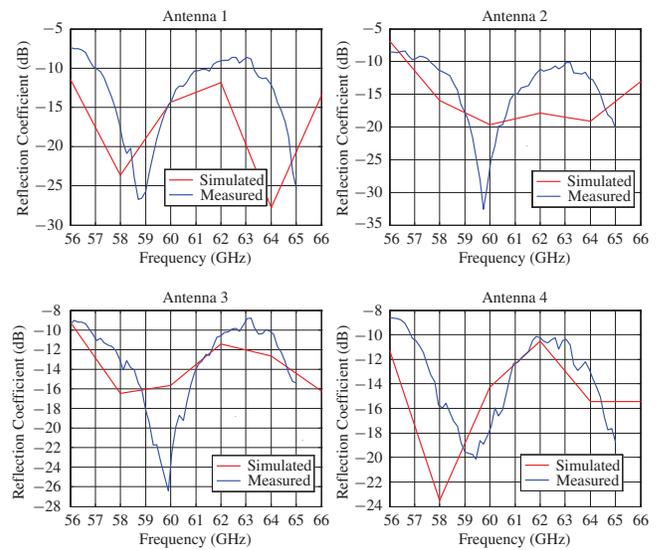
Fig. 10. Comparison of simulated and measured reflection coefficients, antennas 1–4 of Rx package.
