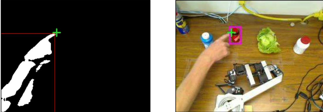
**Fig. 7.** Gesture recognition is implemented by using background subtraction to track the user’s hand. The most extremal portion of this mask (left) selects one of the objects previously identified (right).
