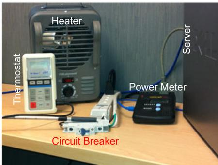
Figure 4: Hardware testbed.
