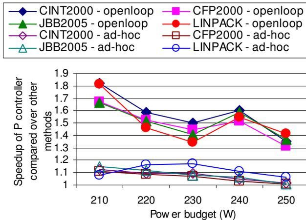
**Figure 10: Speedup of P controller over other methods.**
