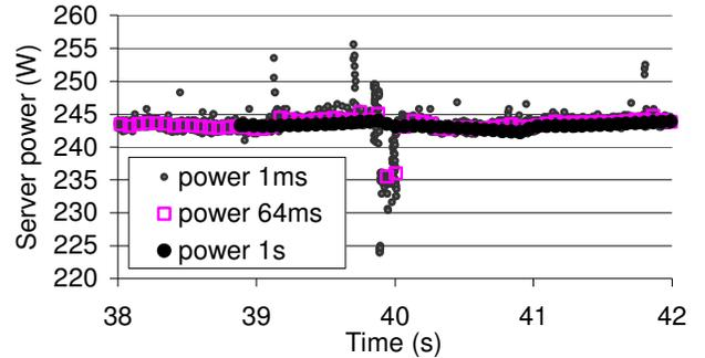
**Figure 6: Linpack without power management.** Graph shows 4 seconds of the Linpack benchmark after running for 38 seconds. Average power over 1 ms, 64 ms, and 1 s periods is plotted. The plot points mark the end of the measurement period. Linpack has almost constant power consumption with periodic dips in power (as seen around the 40 second mark).
