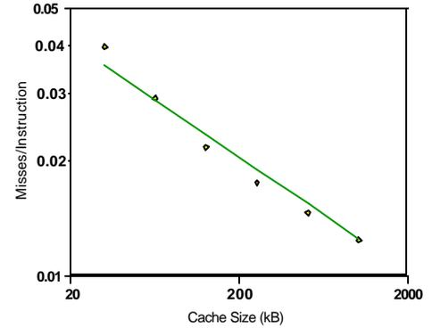
Fig. 7 shows the cache miss rate as a function of cache size for an L2 cache using OLTP-1
