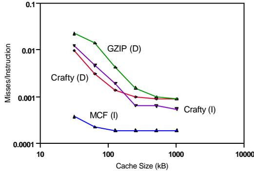
Fig. 8 shows the variation of cache miss rate with cache size for some SPEC workloads. Saturation for large caches is clearly observed.
