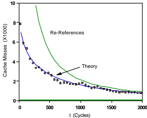
Fig. 3 shows the cache misses as a function of the re-reference time for a direct mapped cache and the OLTP-1 workload.
