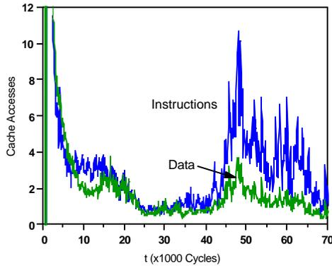
Fig. 9 shows the cache re-reference pattern for the simulator workload. The large peak for both data and instructions is clearly evident.
