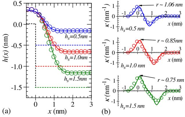
FIG. 2 (color online). (a) Graphene geometry  $h(x)$  for various step heights as indicated. Symbols are the full numerical calculation. Solid lines are best fit using Eq. (1). The respective step profile are illustrated by dashed lines. (b) Corresponding curvature  $\kappa$  for geometries shown in (a), with lines and symbols as in (a). The minimum radius of curvature (inverse of maximum  $\kappa$ ) is indicated.
