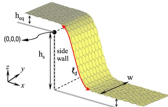
FIG. 1 (color online). Illustration of graphene over a substrate step. Here  $h_s$  is the step height and  $h_{\text{eq}}$  is the equilibrium distance of graphene from the substrate surface due to van der Waals interaction.  $l_d$  is the length of graphene detachment from the substrate.
