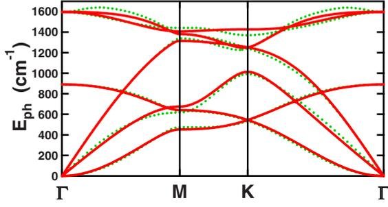
FIG. 1. (Color online) Phonon band dispersions. Green dotted curves are LDA calculations (Ref. 7). Red solid curves are results of the model [Eq. (1)] fitted to these LDA calculations. The corresponding parameters are given in Ref. 16.
