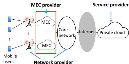
Fig. 1. Providing services to mobile users via MECs.
