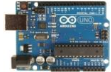
Arduino UNO SDK uses C++ Provides 32k Flash
